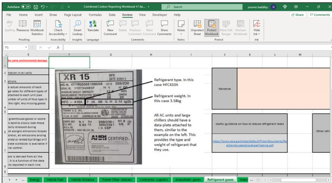
These data plates should state the type of refrigerant and the weight of refrigerant normally held in the equipment. Alternatively, you may have bottles of refrigerant stored onsite, purchase records, or the engineers that service your equipment may have records of refrigerant used.
